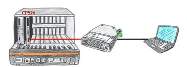
Your visualisation-software does not support a 3964R-protocol, but you have to apply this package? No problem, connect the 3964R-LAN to your CP and activate the RFC1006-emulation in the module. Now your software gets the data from the module via RFC1006, which in turn communicates with the assembly via 3964R.
