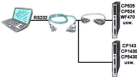
You have a PC with programming software and a 9pin COM-port as interface? No problem, for this purpose the PG-UNI-II-cable is exactly the right product. Connect it to a Siemens assembly such as H1-CP (CP1430), WF470 and PC or CP-525 with the CP525-adapter and PC and you're Online.
