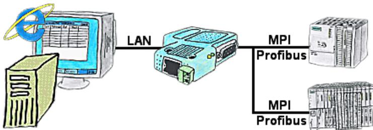
You would like to give your customer the opportunity to read current numbers of the manufacturing Online, without installing a visualisation or even the STEP7-package? Then a S7-LAN with the option Status Variable" is needed, and your customer can take a look at these password protected data on a site of the integrated webservice.
