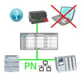
Via digital input triggered DB-backup/-restore without additional PC via PN-port to USB-stick
