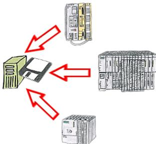
You shortly need a logging of your PLC's operating states respectively are on the way of figuring out a problem and have no datalogger? No problem, connect the PC, start the PG-2000-software with "option datalogger", define relevant variables, appoint timestamp and then the recording starts running immediately. The data will be stored on the fixed disc according to the configuration.
