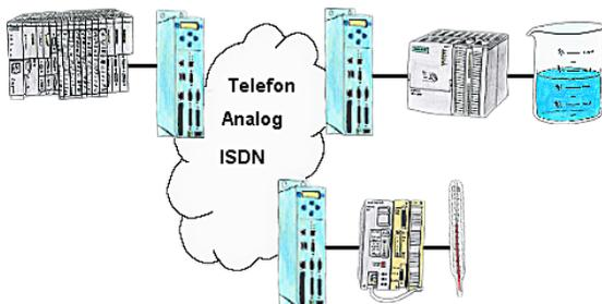
Your pumping stations report the water levels of the central control via telephone network. The central office itself can of course transmit commands/messages to the substations as well. Thereto no dedicated line is required, a "normal" telephone connection is sufficient because the devices cut the line after occurred message.
