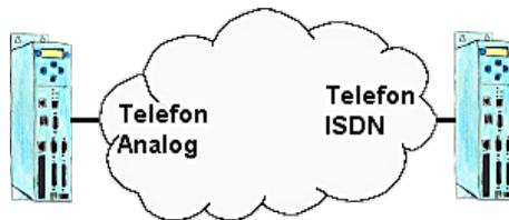
You have on the plant side only ISDN for telephone, but in your office there is only an analogue system? No problem, you have to install on the clients side the TP-II and activate there the analogue-emulation in the device. No, the modem signals will be send digitalized over ISDN and you can connect to it. So, you will be able to communicate though the telephone systems are different and your client isnt forced to install an analogue connection.
