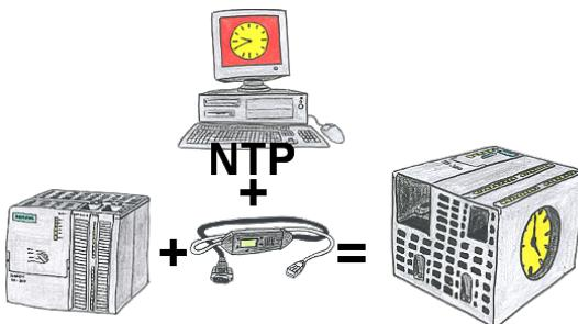
You need in your PLC a actual time? No problem, with the NTP-function the MPI-LAN-cable get from a NTP-(Time-)Server the actual time and transfers it direct into the configured PLC or for processing in a DB.
