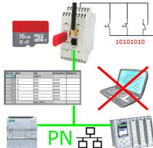
Via digital input triggered DB-backup/-restore without additional PC via PN-port to SD-card
