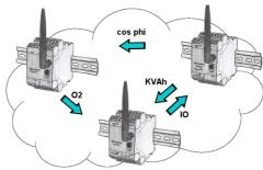
By the EtherSens-cloud each EtherSens-device can exchange data, transfer data and forward to other devices. As if you use one device that records all necessary parameters centrally.
