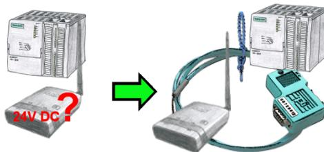
You want to install your ALF directly in the switch-board and would like to use the 24V of the existing S7-PLC? No problem, connect the open ended side of the Kabelbrücke to the 24V port on your ALF and the bus-side on the MPI- or Profibus of this PLC. Even the ALF is supplied above this PLC.
