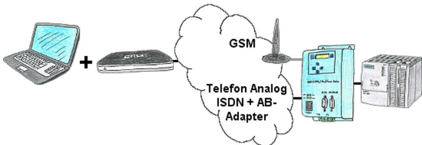
The access to the connected PLC with the Siemens TS-software or PG-2000 including TS-option results of coupling via Analogue-, ISDN- (only with AB-adapter) as well as GSM-line.
