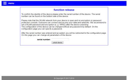
After you have entered the serial number the device is unlocked and can be used normally. To be able to customize the configuration directly, you will be redirected to the configuration page (see picture on the left) after entering the serial number. We recommend that you check and maybe customize the configuration.
