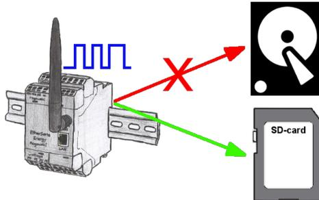
With the integrated SD-card-slot you back-up the recorded data in the device and don't need an external memory. Nevertheless you can send additional the data via FTP to a FTP-server.
