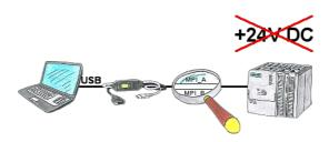
PLC-access in the production-system to "passive assemblies" such as frequency-converter or ET200 or on a bus-connector without PLC, not actually possible without 24V DC for the interface product.
