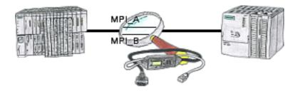
The S7-LAN can also be used for controlling/checking the MPI/Profibus. It will be plugged on the Bus so that you can take a look at the status of the busses via software on PC, for example the numbers of parity errors.
