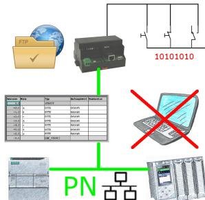
Via digital input triggered DB-backup/-restore without additional PC via PN-port to FTP-server
