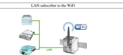
You also need to network devices but dont have locally no ethernet-cable. Wifi is available? With the EtherSens-Bridge you bring immediately all connected wired participants in the WLAN network.
