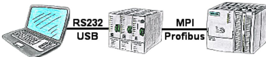
With the TeleService-device you can connect serial or by USB-cable to your PC/laptop and then communicate directly with the control without a PC-adapter or other S7-programming cables.
