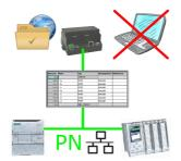
S7-PLC triggered DB-backup/-restore without additional PC via PN-port on FTP-server
