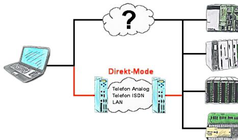
There is an unsupported control or data logger or converter integrated in your installation which protocol is not supported? No problem, the signs that the PC in the office sends will be transferred via telephone line by the Direct-mode, and on-site reproduced by the TP-II. The way back is identical. So in that case there's also a communication to the electronic devices available.
