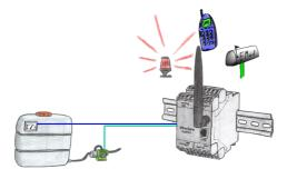
Apply small control tasks of your systems with EtherSens-Control-devices. Determine switching points where the device is running to respond. Depending on the parameterization, an email or SMS notification (depending on the device-configuration) or the device automatically controls via the optional IO-modules (analog / digital / relay).
