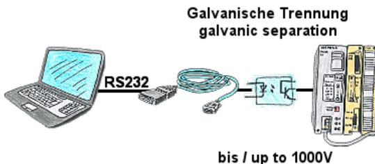
S5-PLC-communication, high-quality PC and fear of interfaces, unsure whether the PLC is grounded or the PLC is in an unsafe environment. Galvanic-separation is the most practical solution. "PG-ISO-Set" (PG-UNI-cable + PG-ISO-adapter) galvanically separates the coupling to the connected S5-PLC, offers protection of the PCs up to a voltage difference of 1000V.
