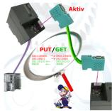
Direct data-exchange between S7-PLCs with S7-LAN.
