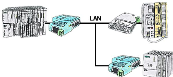
Your pumping stations report the water levels of the central control via telephone network. The central office itself can of course transmit commands/messages to the substations as well. Thereto no dedicated line is required, it's sufficient when the stations connect via network (DSL-router).
