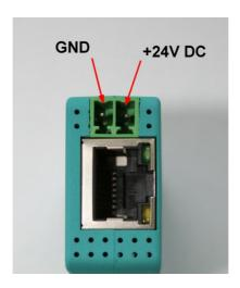
Before using the external supply, check the assignment of the Phoenix connector! The module itself is protected against polarity reversal, but this cannot be guaranteed if it is attached to another module.
