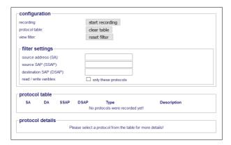
The recording is started with "start recording". Similarly, the stop button "stop recording". "Clear table" deletes the log table for a recording. The same can be achieved by leaving the menu and reopening it.
