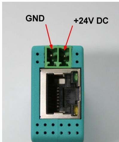
**Before using the external supply, check the assignment of the Phoenix connector! The module itself is protected against polarity reversal, but this cannot be guaranteed if it is attached to another module.**
