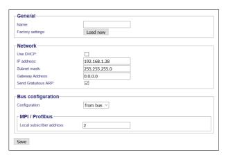
The MPI / DP bus communication analyzer only needs to enter the bus address of the participant whose communication is to be monitored. This is done in the "Observation target address" menu. Otherwise, the bus to be monitored and the network settings are specified here. You can also assign a device name. This is then also visible in the TIC if you are using several devices in the same network.
