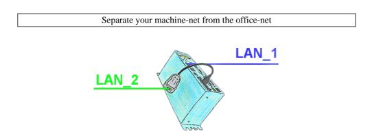
You need a separation between the machine-net and the office-net? No problem, plug a PCMCIA-LAN-card in your Tele-Prof-II-device (only for version -H) and the separation is OK. You have access to both nets via remote maintenance.
