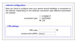
Peculiarity: The APN "internet" is standard for most providers, but can be changed if necessary
