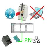
S7-PLC triggered DB-backup/-restore without additional PC via MPI/Profibus on USB-stick
