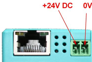
**Before the use of external power supply check the correct pinning of the Phoenix plug! The module itself is protected of wrong pinning of the phoenix plug, but we cannot guarantee for possible connected assemblies.**
