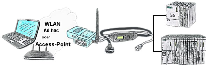
You're right in the middle of your production line and should move around the machine and simultaneously observe / manage. No problem, you parameterize the S7-WLAN-Bridge, connect to the MPI-LAN and connect to an access-point or with the ad-hoc-network of your laptop and are ONLINE on the PLC.
