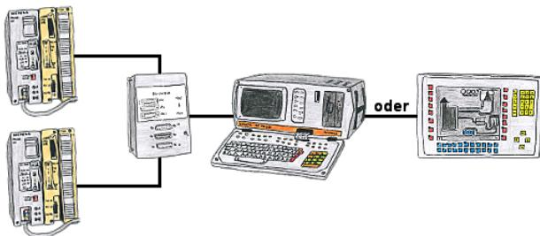
You have to work with more PLC-devices, but no pleasure to switch on/off? No problem, you connect a device of the AG-Switch-family to the PLC-devices and your PD/PC and you will be able to communicate to both PLCs. The selection which PLC you make for AG-Switch-I via toggle switch and for the AG-Switch-II via 24V-controll input.
