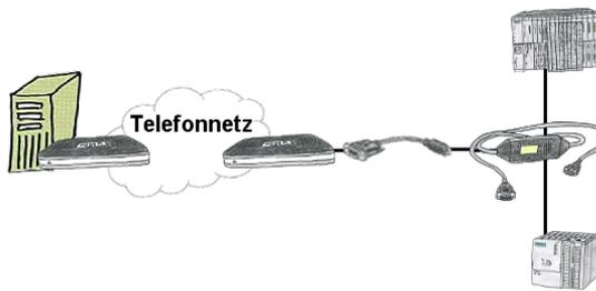
You have to reach urgent your PLC via remote maintenance and have no TS-adaptor in your company? No problem, configure with the MPI-Kabelmanager your S7-interface-cable MPI-II-Kabel the mode "TS" for "remote maintenance", connect this cable with the TS-Adapter (article number 9350-TS) with a standard modem and send it all to your client. Now you will be able to start the connection with your TS-software and solve the problem. And this all without buying a original TS-adaptor.
