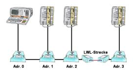
You need for your L1-Bus higher distance like the possible 1200m? You have strong distrubance on your L1-Bus? You need a serial line for higher distances and this galvanic decoupled? No problem, all this points are solved through the LWL-adapter. They are available for artificial and optical fibre, for L1-Bus and RS232.
