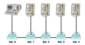
You have to link several S5-PLC's so that in case of need you can respond to all of them without modifying the PLC-program? No problem, connect all PLC's that are in the run with the IBX-Klemme, set up the respective address (1 to 30) at the IBX-Klemme and with the address 0 you will be able to respond to all PLC's via PD-bus-path selection.
