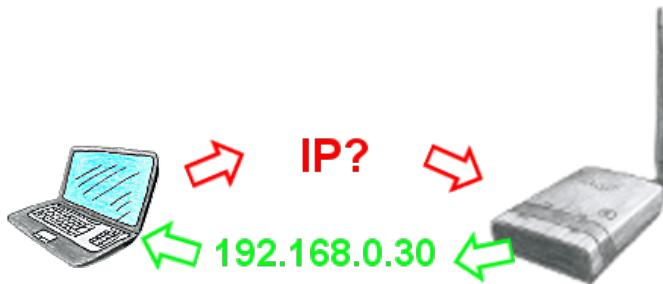
You use your PC in your company network with DHCP, so you dont have to care the everlasting setting of the ip-address. No problem, ALF also can be configured as a DHCP-server and assigns you accessing to the device via LAN or WLAN an ip-address from a predefined address range.
