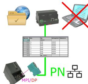
S7-PLC triggered DB-backup/-restore without additional PC via MPI/Profibus on FTP-server
