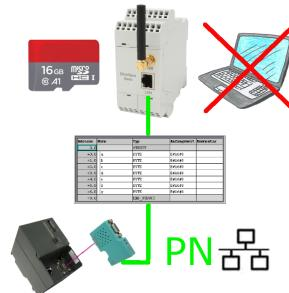
S7-PLC triggered DB-backup/-restore without additional PC via MPI/Profibus on SD-card
