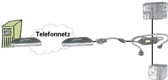
You have to reach urgend your PLC via remote maintenance and have no TS-adaptor in your company? No problem, configure with the MPI-Kabelmanager your S7-interface-cable MPI-II-Kabel the mode "TS" for "remote maintenance", connect this cable with the TS-Adapter (article number 9350-TS) with a standard modem and send it all to your client. Now you will be able to start the connection with your TS-software and solve the problem. And this all without buying a original TS-adapter.
