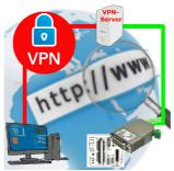
Remote-maintenance of a Siemens-S5-controller with S5-LAN++ on PD-port over separate VPN-server
