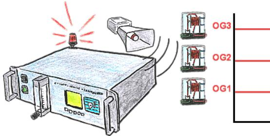
You need some limits? No problem, with the OSC-II-devices you will be able to define 3 relay outputs (toggle switch) like UG (down level) or OG (top level) or as a ready-flag (internal probe has working temperature).
