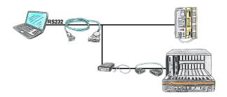
You have a PC with programming software and a 9pin COM-port as interface? No problem, for this purpose the PG-UNI-II-cable is exactly the right product. Connect it to PLC and PC and you're Online. The communication itself is visible by the both included LEDs. Even the 25pin interface of the AS511-card is no problem. You need the NETZ-adapter and also the AG-150-adapter and then this control is programmable, too.
