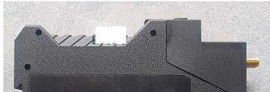
Insert the SIM card with the contact side facing down (slanted corner at the front right) into the slot until it clicks. Pressing again releases the card and it can be pulled out.
