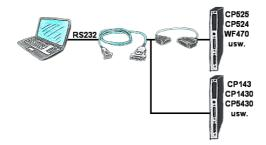
You have a PC with programming software and a 9pin COM-port as interface? No problem, for this purpose the PG-UNI-II-cable is exactly the right product. Connect it to a Siemens assembly such as H1-CP (CP1430), WF470 and PC or CP-525 with the CP525-adapter and PC and you're Online.
