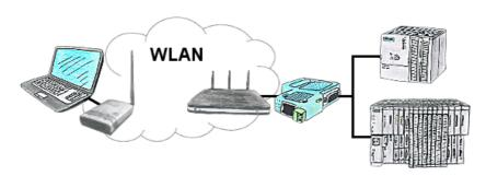
You are on site your plant and should move round the machine and simultaneously control or monitor. WLAN is reachable, but your PC is not able to provide WLAN. No problem, you parametrize ALF as a client and connect him to the PC and join the reachable WLAN and you are online on the PLC.
