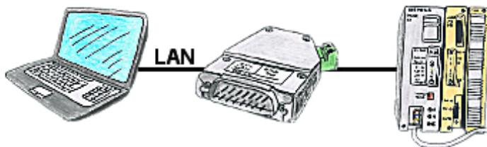
You would like to respond to your S5-PLC via LAN, but not integrate an Ethernet-CP? No problem, plug the S5-LAN++ on the PD-interface and access via LAN.
