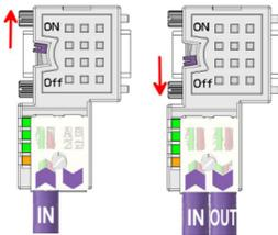
The switchable terminating resistors are activated by a slide switch, easily accessible from both sides right and rear.
