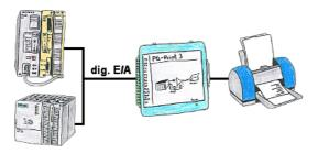
You need production data, circulation lists of your PLC's, but don't want to use a CP or don't get a serial printer anymore? No problem, you need 8 digital outputs and 3 digital inputs of the PLC, and if you connect the PG-Print at it you can generate these lists with a EPSON- or HP-compatible parallel printer.
