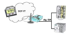
For your production flow you're always in need of an exact time? No problem, connect the SPS-Clock with 4 digital in-/outputs of your PLC, after synchronisation of the SPS-Clock the updating time can be read in a DB of the PLC.
