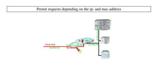
You have in your facility machines from different manufacturers and no one does get access to the controls of the other? No problem, with the S7-firewall you can filter who can ever communicate with the control network and which user with which end users. This is done through the IP address and MAC address.
