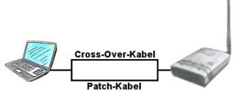
You need ALF to connect to a reachable WLAN, but only have a patch-cable? No problem, ALF provides "autonegotiation" and this means that he recognises a connected cable (patch-cable or cross-over-cable) and surround the pinning according to the cable, so a communication is possible.
