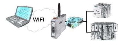
Your're right in the middle of your production line and and should move around the machine and simultaneously observe / manage. No problem, you parameterize the ALF, connect to the S7-LAN and connect to the WIFI-network of the ALF and are ONLINE on the PLC.
