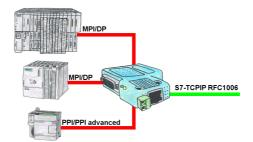
Networking of all S7-controllers (S7-200/300/400), for example with your production-data-acquisition, Industry 4.0 (OPC Server UA or Classic), panels and other devices that communicate via S7-TCPIP RFC1006. One module for all bus-types: PPI, MPI and Profibus.
