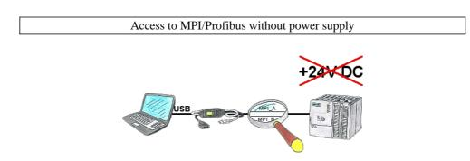
PLC-access in the production-system to "passive assemblies" such as frequency-converter or ET200 or on a bus-connector without PLC, not actually possible without 24V DC for the interface product.
