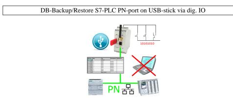
Via digital input triggered DB-backup/-restore without additional PC via PN-port to USB-stick
