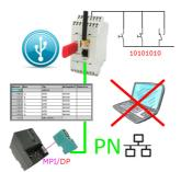
Via digital input triggered DB-backup/-restore without additional PC via MPI/Profibus to USB-stick
