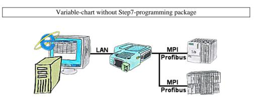
You would like to give your customer the opportunity to read current numbers of the manufacturing Online, without installing a visualisation or even the STEP7-package? Then a S7-LAN with the option Status Variable" is needed, and your customer can take a look at these password protected data on a site of the integrated webserver.
