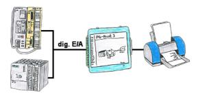
You need production data, circulation lists of your PLC's, but don't want to use a CP or don't get a serial printer anymore? No problem, you need 8 digital outputs and 3 digital inputs of the PLC, and if you connect the PG-Print at it you can generate these lists with a EPSON- or HP-compatible parallel printer.
