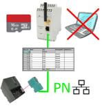
S7-PLC triggered DB-backup/-restore without additional PC via MPI/Profibus on SD-card
