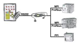
Your panel provides a serial port and no MPI/Profibus for connecting a S7-PLC. Connect the MPI-II-cable with it and you're Online with your panel.
