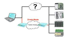
There is an unsupported control or data logger or converter integrated in your installation which protocol is not supported? No problem, the signs that the PC in the office sends will be transferred via telephone line by the Direct-mode , and on-site reproduced by the TP/TB. The way back is identical. So in that case there's also a communication to the electronic devices available.
