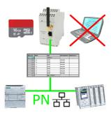
S7-PLC triggered DB-backup/-restore without additional PC via PN-port on SD card
