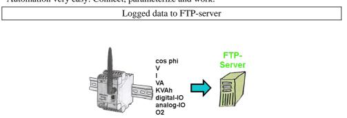
Do you need the logged data not locally but on your site? Then just turn on recording on an FTP-server and the data is stored. You can then immediately read and process this data.
