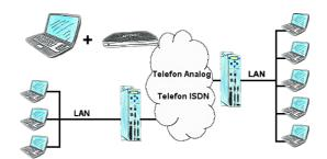
The Tele-Prof-II can also be used as a router for access from a PC via dial-up connection, so that a communication with the behind covered network results. Furthermore a network connection can be made with the TP-II TP-II-line, but in doing so the IP-address-root must differ.
