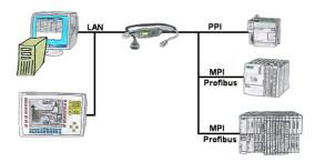
Your panel only has a LAN-socket as PLC-interface? No problem, connect this socket with the S7-LAN or the MPI-LAN-cable and plug it directly on the PPI/MPI/Profibus of the PLC. Then access to the variables and data of the PLC is already available.
