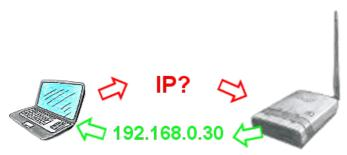
You use your PC in your company network with DHCP, so you dont have to care the everlasting setting of the ip-address. No problem, ALF also can be configured as a DHCP-server and assigns you accessing to the device via LAN or WLAN an ip-address from a predefined address range.
