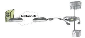
You have to reach urgend your PLC via remote maintenance and have no TS-adaptor in your company? No problem, configure with the MPI-Kabelmanager your S7-interface-cable MPI/PPI-Kabel the mode "TS" for "remote maintenance", connect this cable with the TS-Adapter (article number 9350-TS) with a standard modem and send it all to your client. Now you will be able to start the connection with your TS-sofware and solve the problem. And this all without buying a original TS-adapter.
