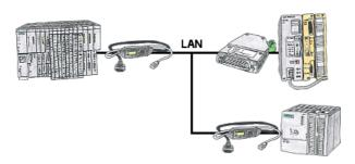
Your pumping stations report the water levels of the central control via telephone network. The central office itself can of course transmit commands/messages to the substations as well. Thereto no dedicated line is required, it's sufficient when the stations connect via network (DSL-router).
